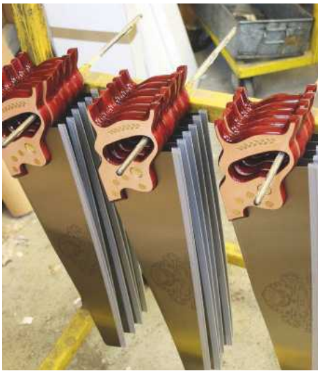
▲ Hand-lacquered and sprayed handles on the top-end saws give them a classy look to match their performance
